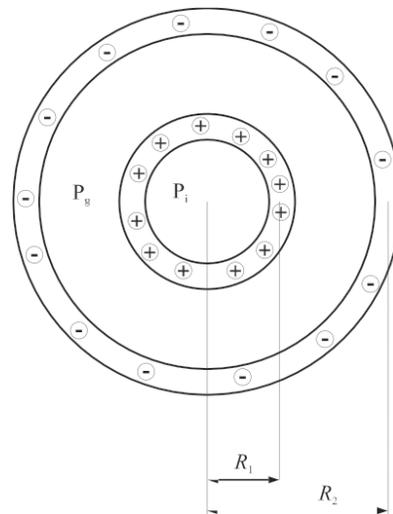
**Figure 4. The atmospheric spherical capacitor.  $R_1$  and  $R_2$  are average radii of the inner and outer bubbles respectively.  $P_a$  is atmospheric pressure,  $P_g$  is pressure in the gap, and  $P_i$  is the pressure in the inner bubble.**
