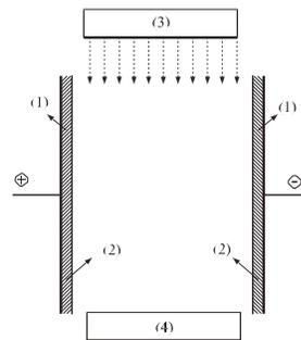
Figure 5. A schematic sketch of apparatus simulating conditions for generation of ASC. A planar capacitor (1), a dielectric layer (2), a source of ionizing radiation (3), and a source of plasma (4) are basic elements of the apparatus.
