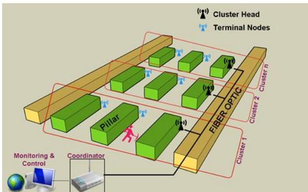
**Fig. 1** The cluster-tree topology of a mine site
