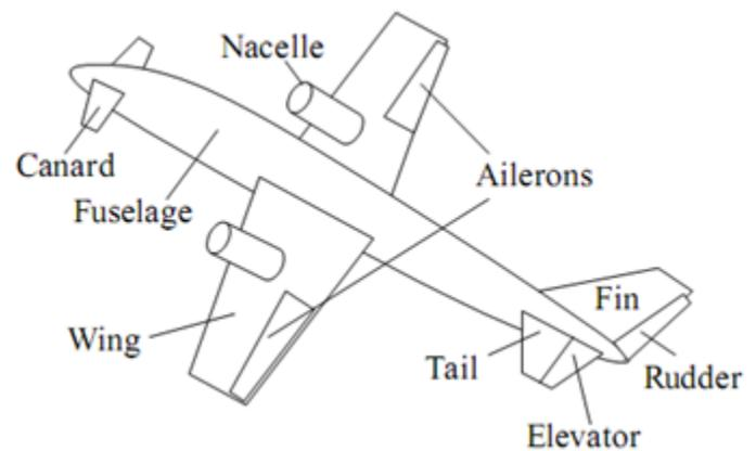
*Fig.1. Elements of Airplane Configuration*
