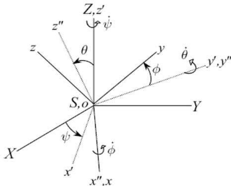
Fig.4. The Orientation of Aircraft Axes, (oxyz), Relative to Ground Station, (SXYZ)
