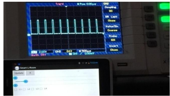
Fig:16 Test of Dim Light with PWM (Low Brightness)
