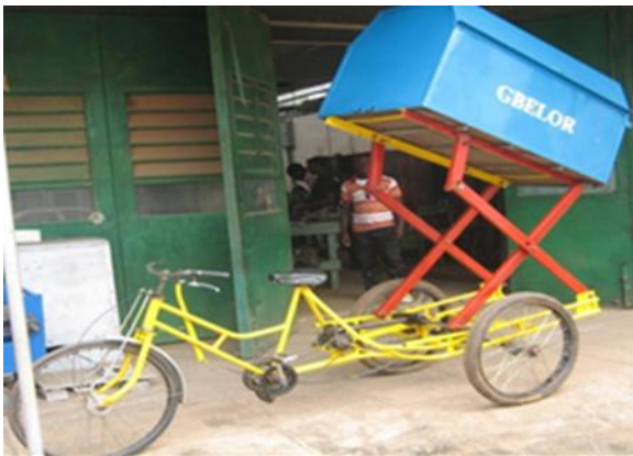
Figure 1: Tricycle with tipping mechanism at full tipping position
