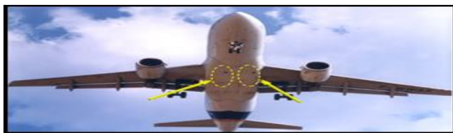
Figure(2-3): two air conditioning packs located in the wing root
