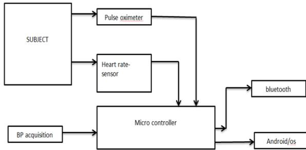
The signal accession unit comprises of the two different sensors spo2 sensor and the heart rate sensor, here we used Max30100 and HW01 sensors for acquiring the respective parameters. The microcontroller used here is arduino UNO (ATmega328P) which is programmed for the signal processing and the display system used is LCD.
