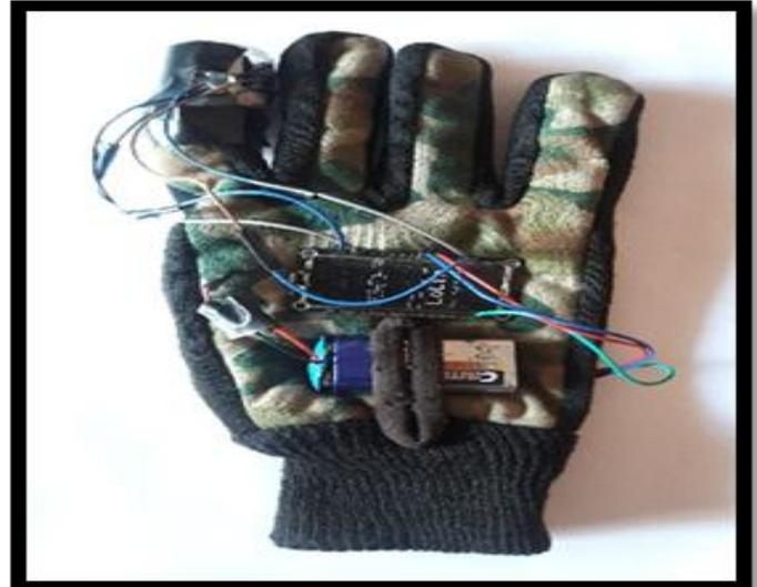
FIG. 2. HAND WITH SENSORS AND CONTROLLERS
