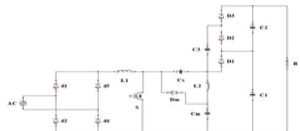
**Fig.2.2** Switch OFF mode of Modified multiplier SEPIC PFC topology
