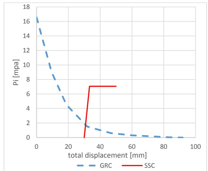
**Figure 5:** Ground reaction curve (GRC) and Support characteristic curve (SCC) plotted in same graph to determine stability of tunnel section against squeezing.
