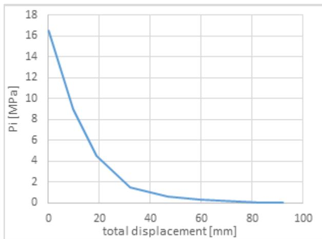
**Figure 4** Ground responsive curve for tunnel section at 2+500m
