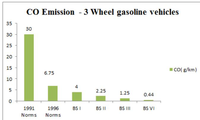
**Fig. 9.** Maximum Allowable CO emission from 3 wheeled gasoline powered vehicles according to various emission standards of India
