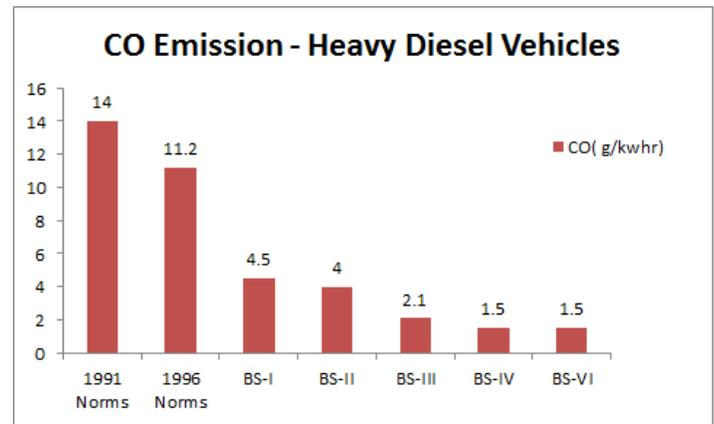
**Fig. 5.** Maximum Allowable CO emission from Heavy Diesel Vehicles according to various emission standards of India.
