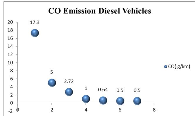
**Fig. 2.** Maximum Allowable CO emission from passenger cars powered by diesel according to various emission standards of India
