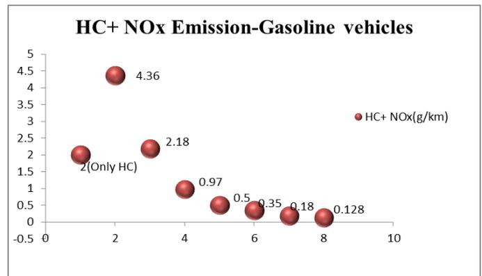
**Fig.3.** Maximum Allowable HC+NOx emission from passenger cars powered by petrol according to various emission standards of India.
