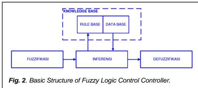
Fig. 2. Basic Structure of Fuzzy Logic Control Controller.
