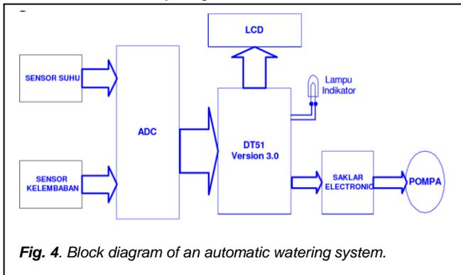
Fig. 4. Block diagram of an automatic watering system.
