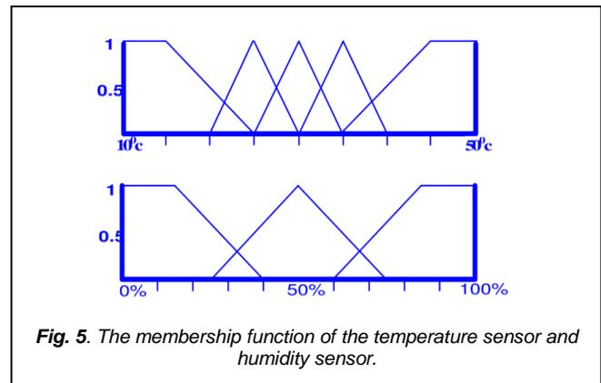
Fig. 5. The membership function of the temperature sensor and humidity sensor.
