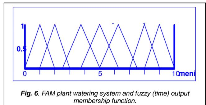
Fig. 6. FAM plant watering system and fuzzy (time) output membership function.
