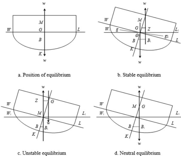
**Figure 1.** Vessel equilibrium (Smith, 1975). B - centre of buoyancy, G - centre of gravity, M - Metacentre, GZ - Righting arm, K - Keel, WL - Water line, w – Force,  $\theta$  - Rolling angle.
