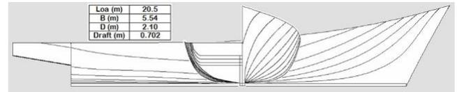
**Figure 3.** Hull line of PKU-2
