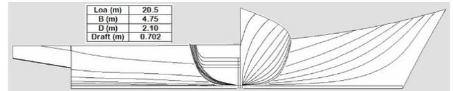
**Figure 4.** Hull line of PKU-3
