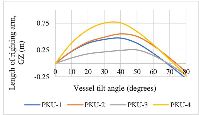
Figure 6. Ship static stability curve at mean load condition.
