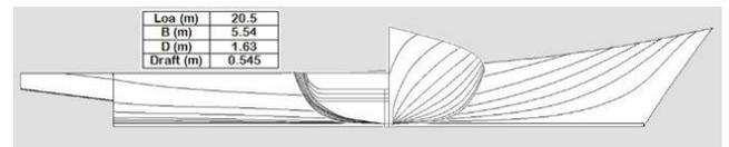
**Figure 5.** Hull line of PKU-4
