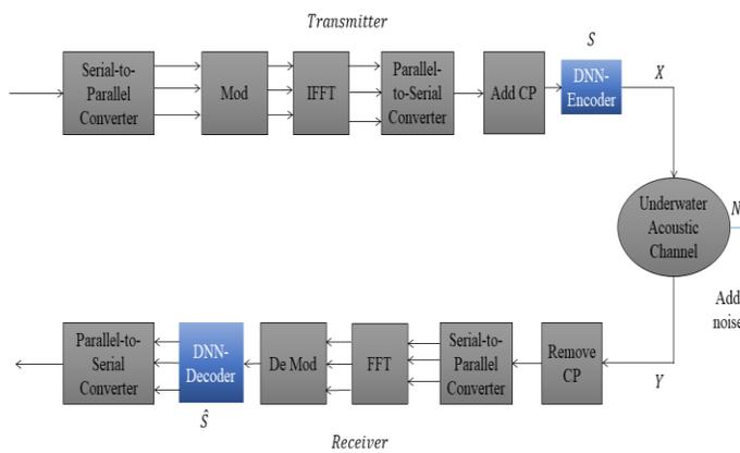
Fig. 1. Block diagram of proposed DNN-autoencoder in UWA OFDM system
