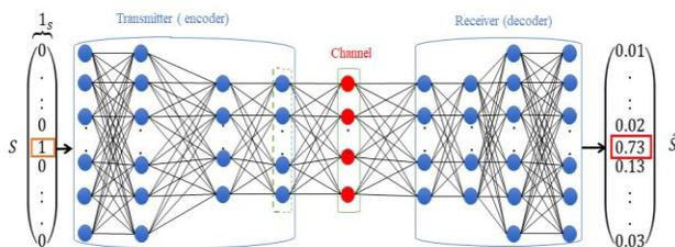
Fig. 2. Proposed PAPR reduction method based on auto-encoder in UWA OFDM system
