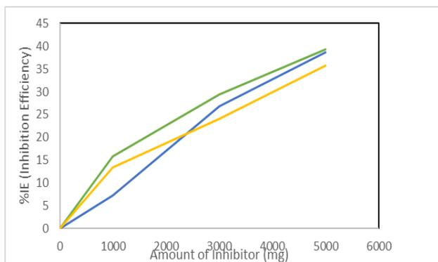
**Fig 4** The correlation between the amount of inhibitor and Inhibitor Efficiency (%IE)
