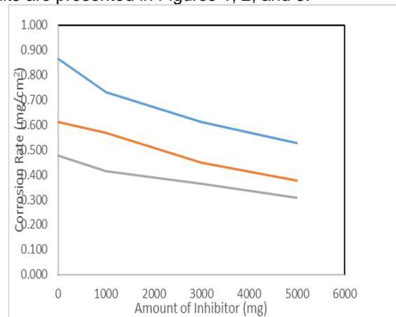
**Fig 1.** The correlation between the amount of organic inhibitor added and corrosion rate
