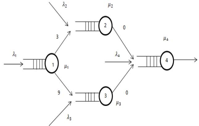
**Fig. 4** Open Queueing Network Model
