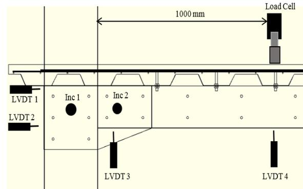
**Figure 5 The Schematic of isolated joint test**
