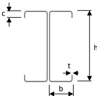
**Figure 3 Double lipped channel profile**
