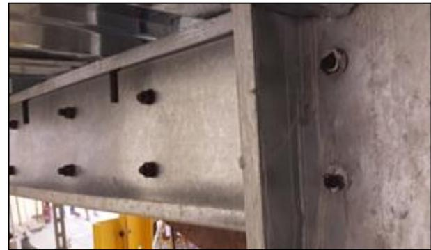
Figure 9 Local buckling of column flange
