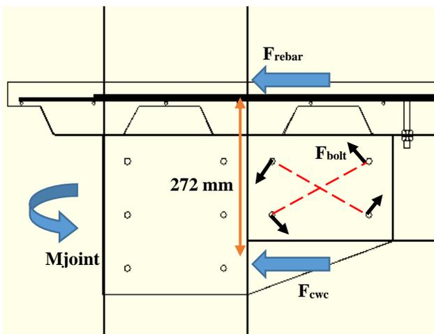
Figure 13 Analytical of moment capacity of joint
