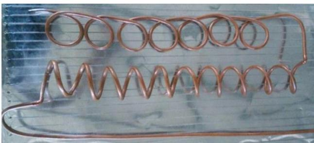
Fig. 1. Heating coil arrangement (Slinky+Spiral+U-type)
