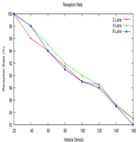
**Fig 8: Reception rate Vs Vehicle density**
