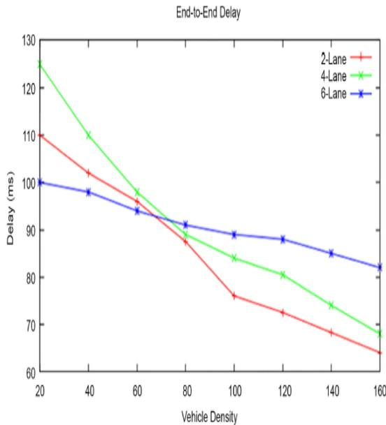
**Fig 7: End to End delay Vs Vehicle density**
