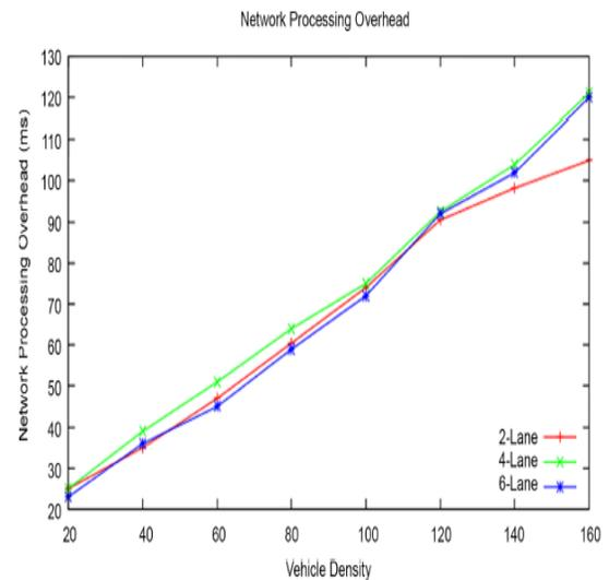
**Fig 9: Network overhead Vs Vehicle density**
