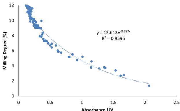
**Fig. 5.** Model of DM by gravimetry relationship with UV absorbance characteristic values
