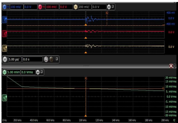
Figure 4.4 AC line Differential Mode noise
