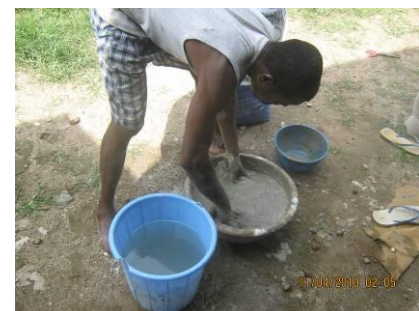
Plate 5: Mixing the 3 constituents of the composite mould with water.
