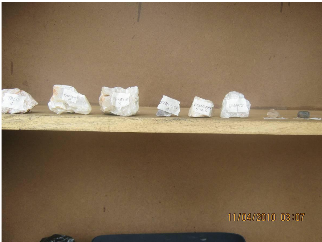
Plate 7: Mohs' scale Minerals used for the hardness determination: from L to R: Talc (1), gypsum (2), calcite (3), fluorite (4), feldspar, (4-7, mean = 5.5), quartz (7), topaz (8) & corundum (9).
