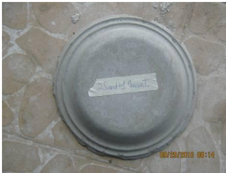
Plate 6a: (2 sand + 1 cement + 0 pop) trial mix cast
