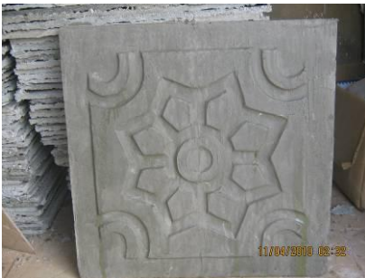
Plate 6c: ( 1\frac{1}{2} sand + \frac{3}{4} cement + \frac{3}{4} pop) mould (600 mm x 600 mm).
