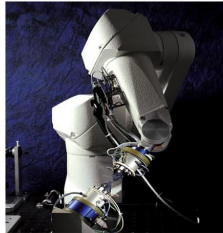
*Figure 5: SureSmile wire bending robot (Orametrix, Richardson TX)[2].*
