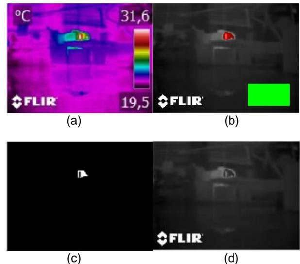
**Fig. 5.** Scenario 4. Frame 1780. (a) Original image, (b) Final result, (c) Thermal binarization, (d) Histogram equalization.
