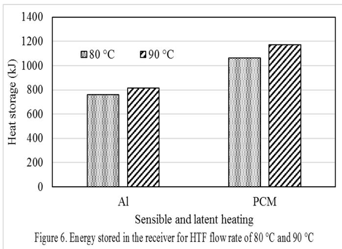
Figure 6. Energy stored in the receiver for HTF flow rate of 80 °C and 90 °C
