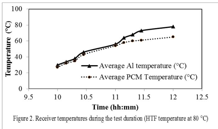
Figure 2. Receiver temperatures during the test duration (HTF temperature at 80 °C)
