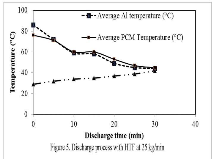
Figure 5. Discharge process with HTF at 25 kg/min
