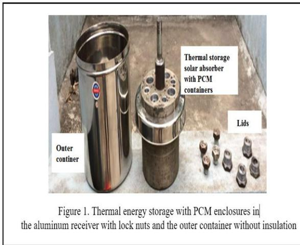
Figure 1. Thermal energy storage with PCM enclosures in the aluminum receiver with lock nuts and the outer container without insulation
