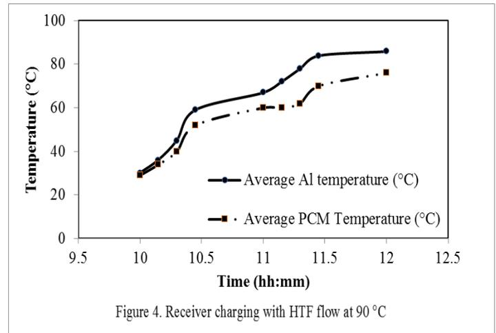
Figure 4. Receiver charging with HTF flow at 90 °C
