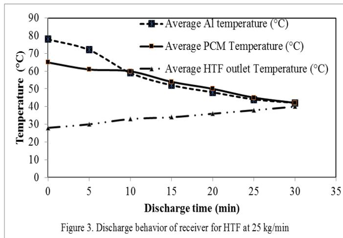
Figure 3. Discharge behavior of receiver for HTF at 25 kg/min
