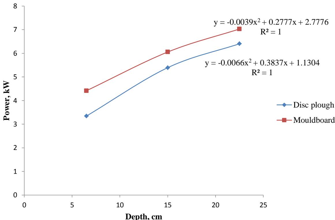
Fig 3.3 Power against Depth for disc and mouldboard plough
