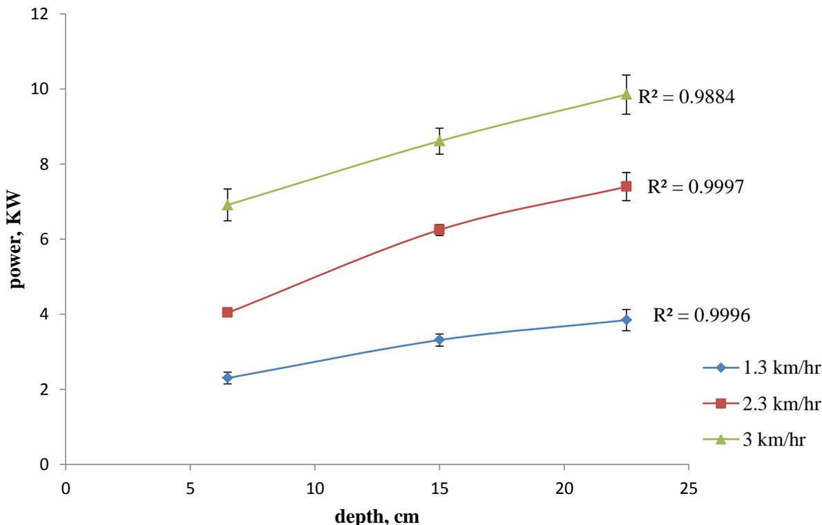
Fig 3.2 Power against depth for mouldboard plough
