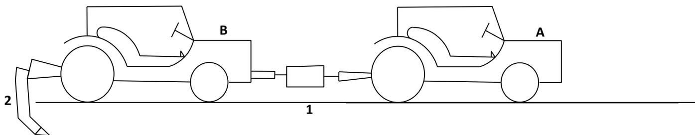
**Fig 2.1** Experimental set-up comprising of two tractors and load cell
