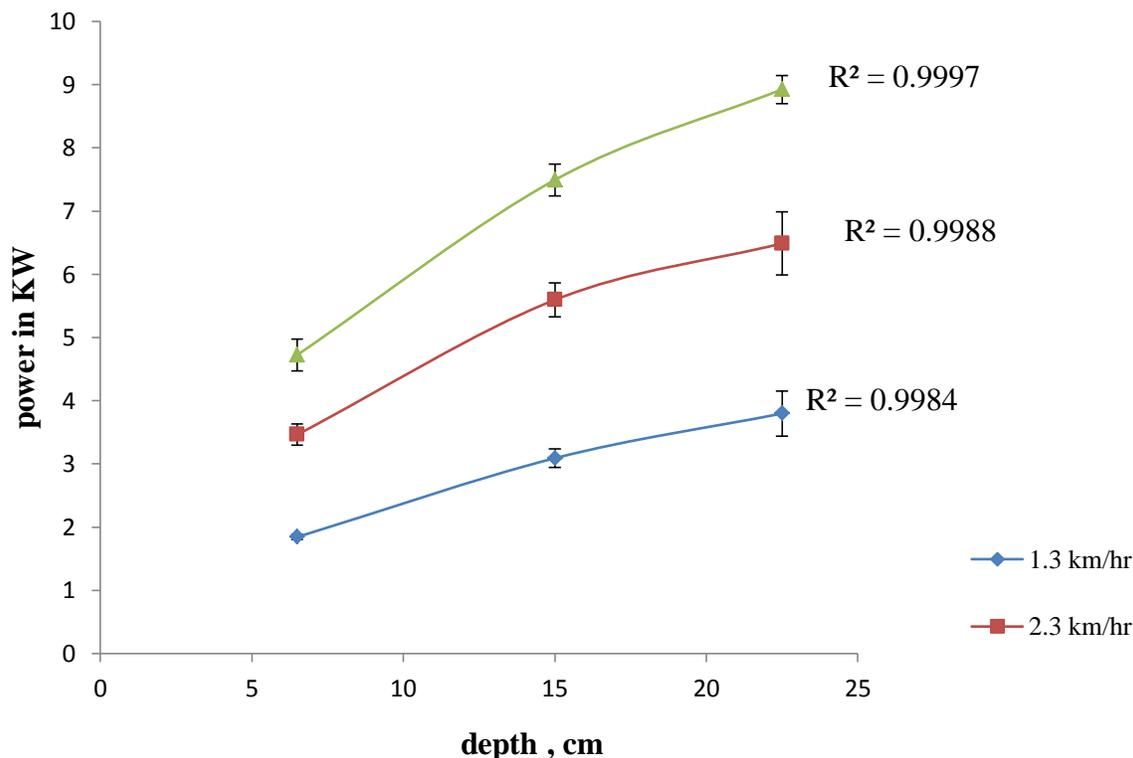
**Fig 3.1** Power against depth for disc plough
