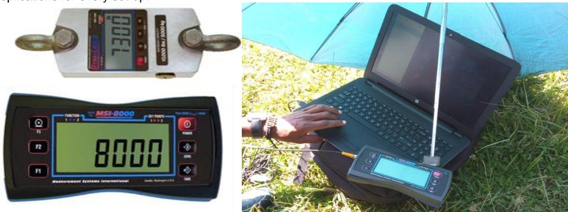
**Fig 2.2** Dyna-Link 2 tension dynamometer set-up (Measuring Systems International 7300)
