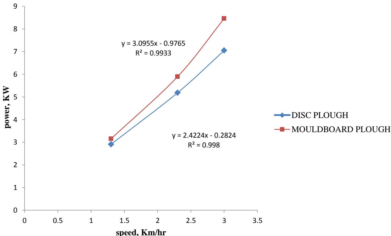
**Fig 3.6** Power against speed for disc plough and mouldboard ploughs
