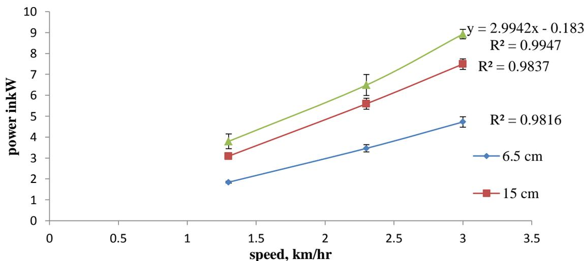
Fig 3.4 Power against speed for disc plough
