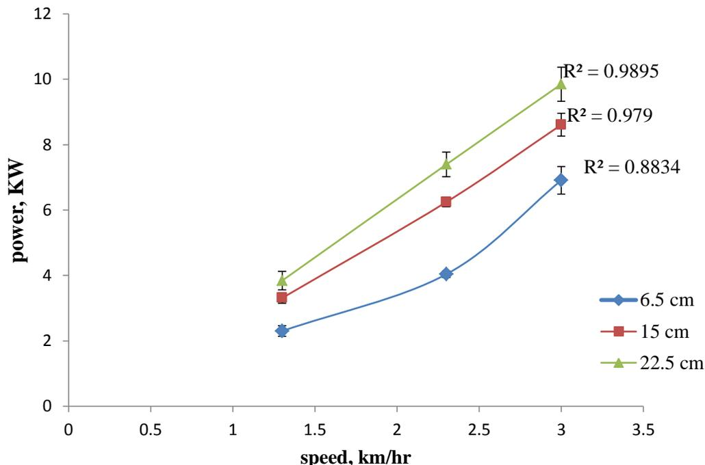
**Fig 3.5** Power against speed for mouldboard plough
