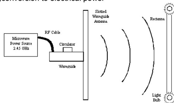
**Fig.4** microwave wireless power transfer technology (MPT)
