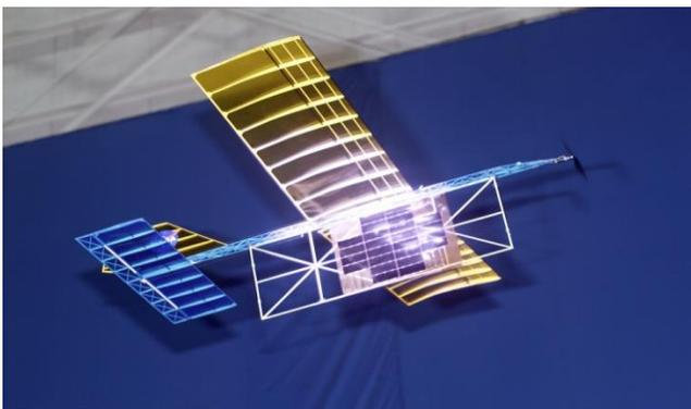
**Fig.5** Laser energy used to power a model airplane with solar cells. Source: [Wikimedia Commons](#) (Courtesy of [NASA](#)).
