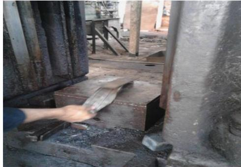
**Fig. 2** Flattenning under hydraulic press
