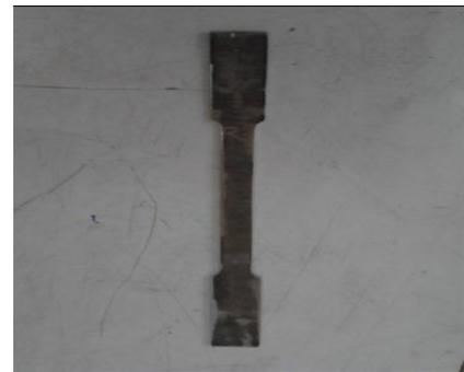
**Fig. 3.** Final shape of the tensile sample extraction from the helmet
