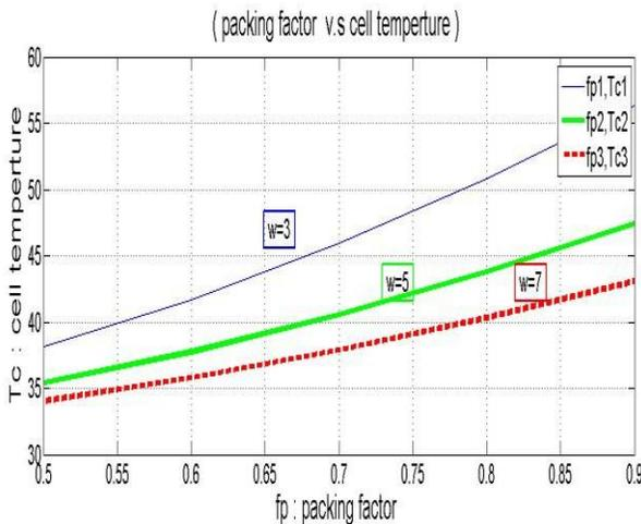
**Fig.5** show the relation between *Fp* (packing factor) and *Tc* (cell temperature) for different values of *w* (wind speed). As seen, one can observe that as packing factor decrease and wind speed increase then cell temperature decreases.
