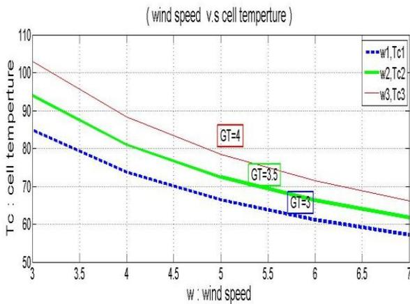
**Fig.4** show the relation between *w* (wind speed) and *Tc* (cell temp.) for different values of *GT* (concentration power). As seen, one can observe that as wind speed and concentration power decrease then cell temperature decreases.
