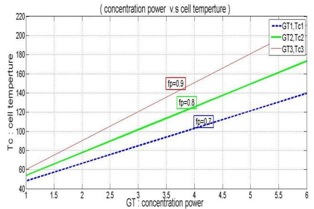
**Fig.6** show the relation between *GT* (concentration power) and *Tc* (cell temperature) for different values of *Fp* (packing factor). As seen, one can observe that as packing factor decrease and wind speed increase then cell temperature decreases.
