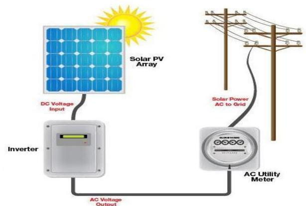
**Fig.7** Block diagram of on grid fixed panels system at  $\beta=30$
