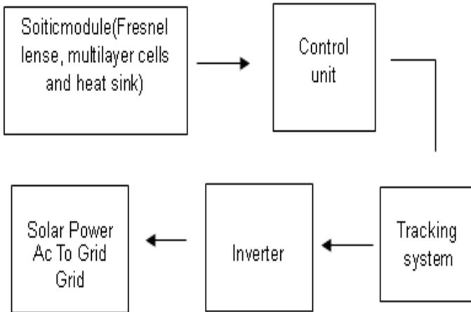
**Fig. (10)** Block diagram of PV system under concentration using soitec module.
