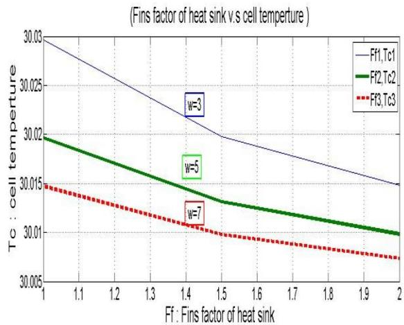
Fig. 3 show the relation between Ff (fins factor) and Tc(cell temp.) for different values of w(wind speed).As seen, one can observe that as fins factor and wind speed increase then cell temperature decreases.
