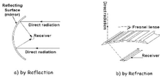
Fig1. Comparison between mirrors and Fresnel lens under concentration. [12]
