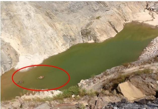
**Fig. 10:** Water pumping to surface from a barge on an open pit sump
