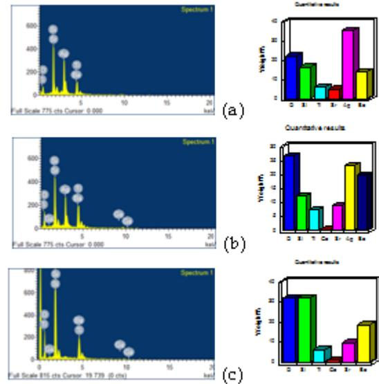
Fig. 4. EDX spectrum of (a) 0 mol% (b) 0.5 mol% (c) 1 mol% Ga doped BST thin films
