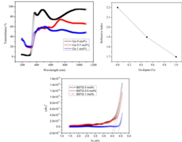
**Fig. 7.** (a) Transmittance (b) Refractive Index (c) Band gap values of BST thin films as a function of Ga concentration.
