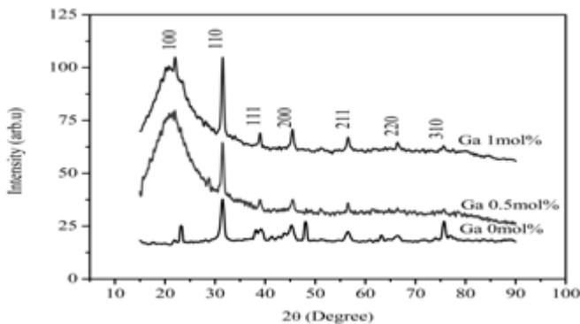
**Fig. 1.** X-ray diffraction of BST thin films for different Ga concentrations.
