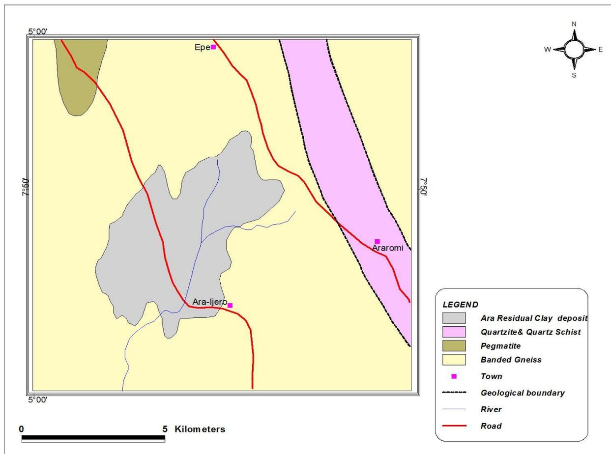
**Fig.2:** Geological map of Ara-Ijero Ekiti showing the Ara Residual clay deposit
