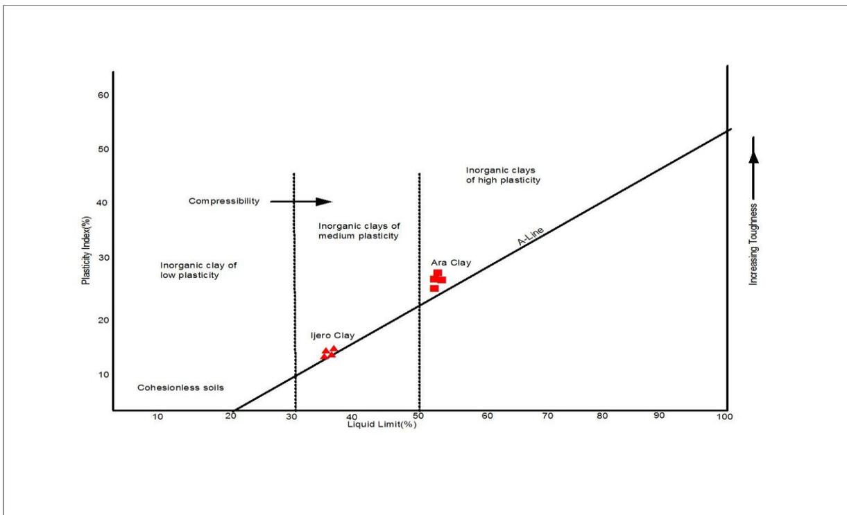
**Fig.5:** Plasticity Chart for the Classification of Ara-Ijero Clay deposit (Casagrande, 1948)
