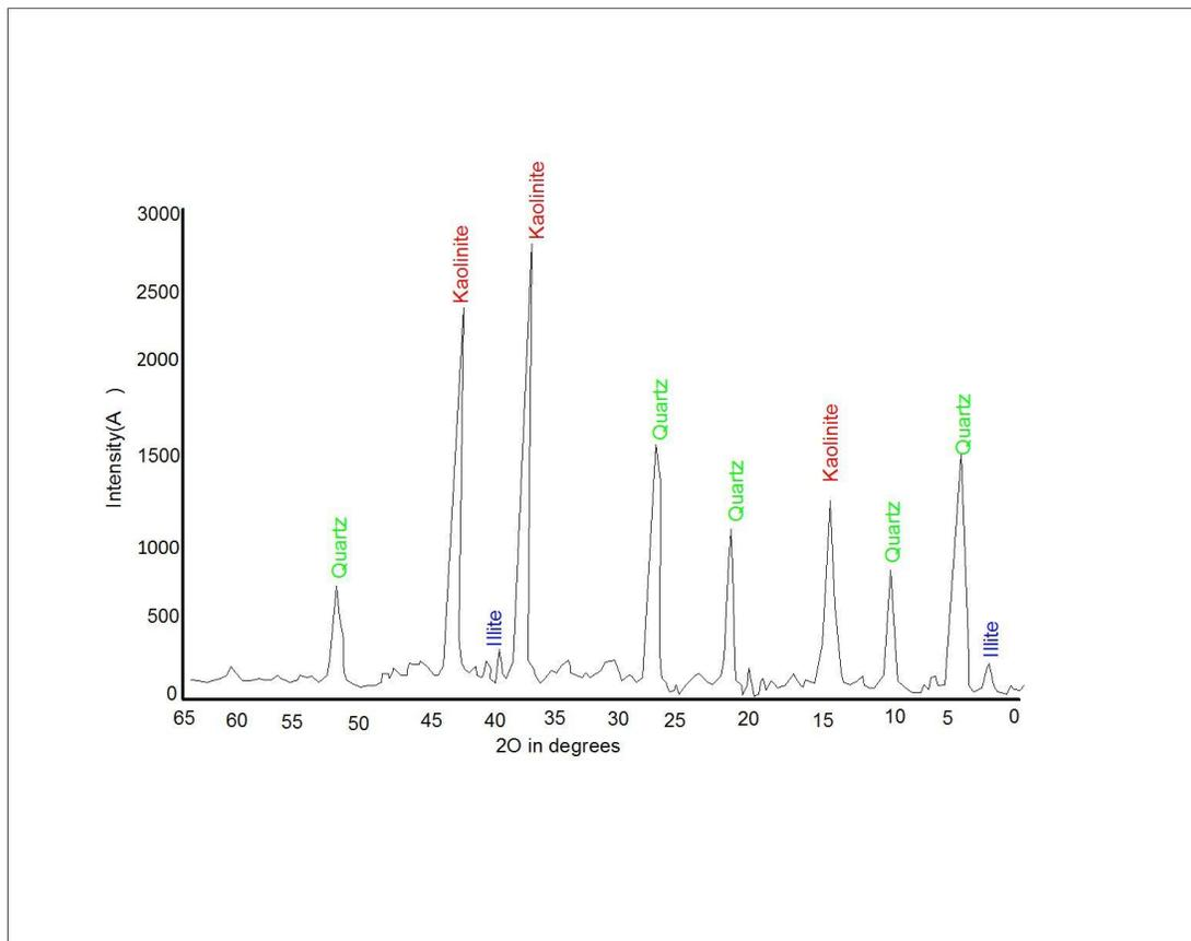
**Fig. 4:** X-Ray diffraction trace of Ara-Ijero Ekiti clay
