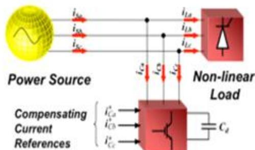
Fig.3 Basic principle of compensator
