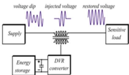
Fig.1 Dynamic voltage restorer
