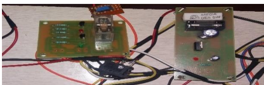
Figure 7 Main Relay with protection circuit.
