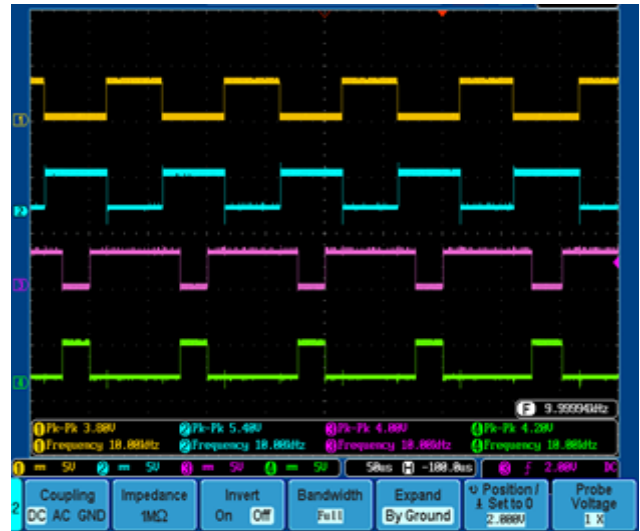
Fig.4 Duty cycles of PWM1, PWM2, PWM5&PWM6.
