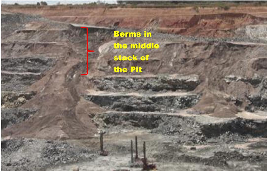
Figure 1. Slope failure recorded in the middle stack of the pit
