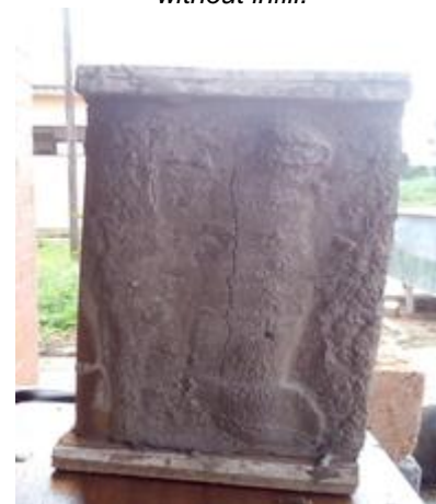
Figure 4: Test setup for compressive strength test for panel with mortar infill
