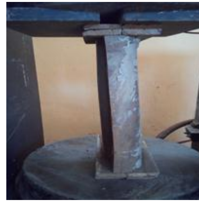
Figure 3: Test setup for compressive strength test for panel without infill.
