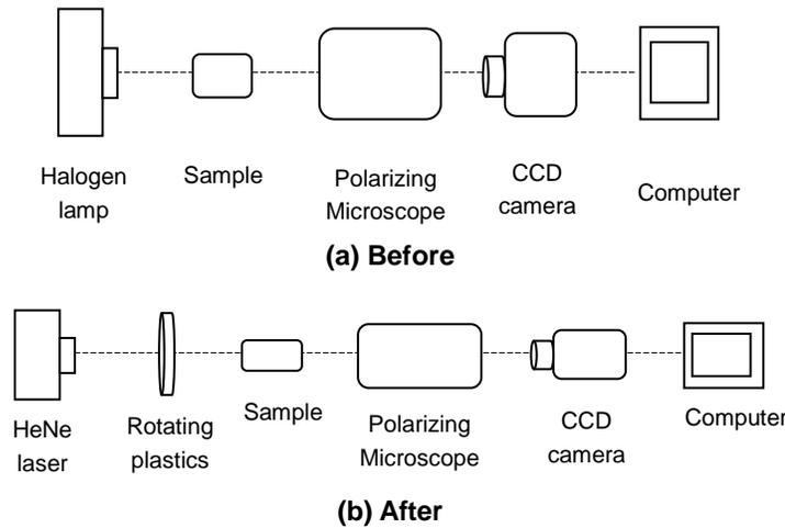
Fig. 1 Schematic illustration of the visibility of domains
