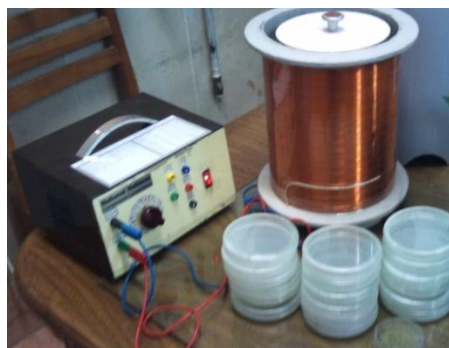
Fig.1 electromagnetic field exposure arrangement
