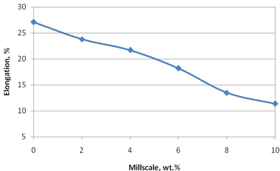
**Fig. 3.** Variation of ductility of aluminium-bronze with millscale content
