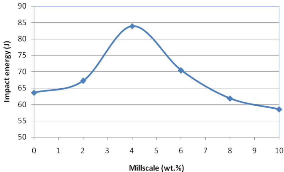
**Fig. 2.** Variation of impact fracture responses of aluminium-bronze with millscale content
