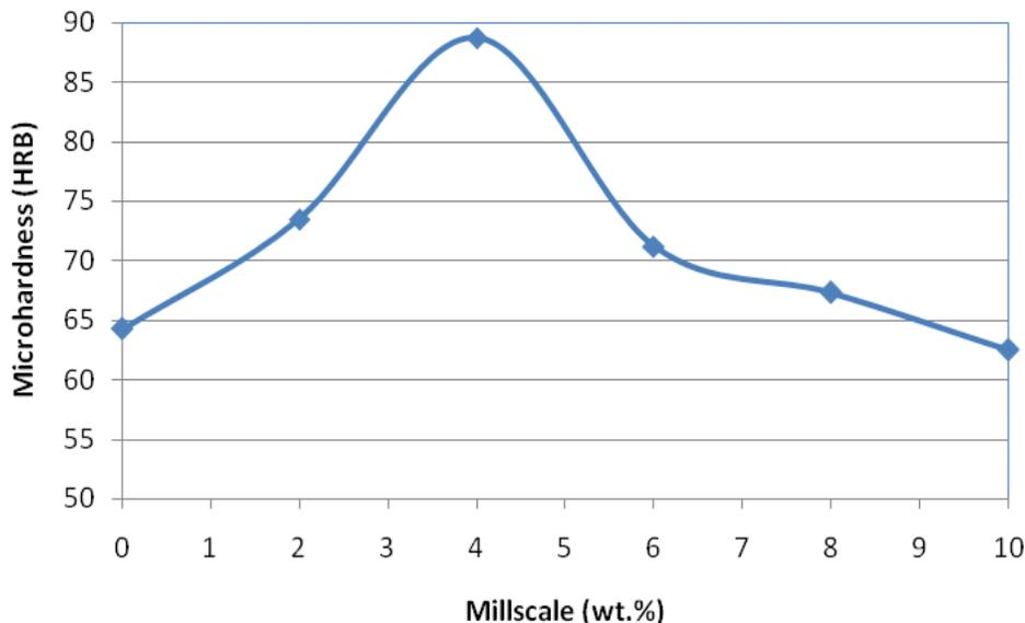
Fig. 4. Variation of micro-hardness of aluminium-bronze with millscale content
