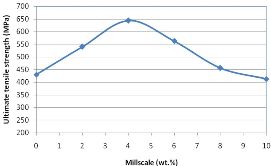
Fig. 1. Variation of ultimate tensile strength of aluminium-bronze with millscale content
