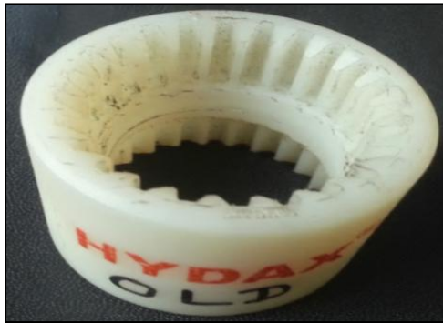
Fig.18 Worn out coupling sleeve
