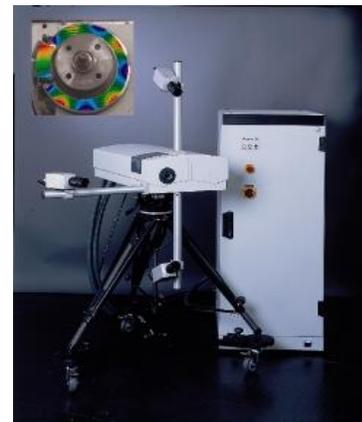
**Figure 3** Dantec Dynamics Company apparatus, 3D Pulse ESPI system, <http://www.dantecdynamics.com/Default.aspx?ID=1603>
